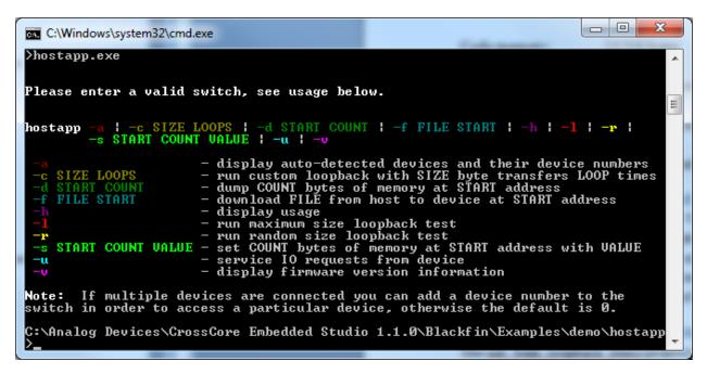
Note: The CLD Bulk Loopback Example supports all of the above command switches except for the '-u' switch.
