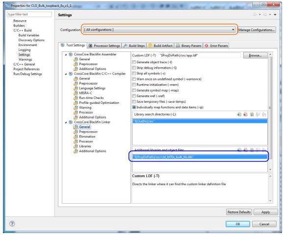
5. The 'Additional libraries and object files' setting needs to be set for all configurations (Debug, Release, etc). This can be done individually for each configuration, or all at once by selecting the [All Configurations] option as shown in the previous figure (circled in orange).
